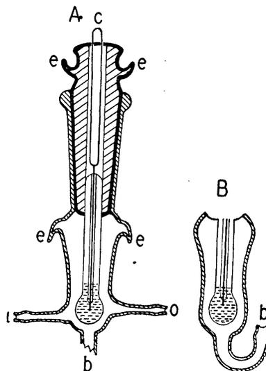
FIG. 1. A, cross section of the glass electrode and chamber, about two thirds natural size; b, position of salt bridge tube; c, wire contact; e-e, glass ears; i, inlet tube; o, outlet tube. B, cross section of the lower part of the chamber, showing the salt bridge tube more in detail. This tube lies in a plane at right angles to the planes of the inlet and outlet tubes.
