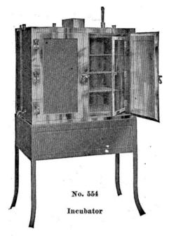
Illustrated is Castle Incubator, Model 554, recommended for milk analysis by the agar plate method. Other models for various bacteriological applications and in various capacities are available. Write:
