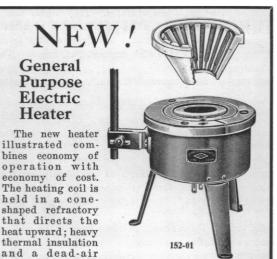
space reduce radiation losses to a minimum. Heating coils are retained in slots in the refractory, deep enough to protect them from me-chanical injury; and replacements are made by lifting the element from the slots, and substituting a new coil. Because the refractory is not discarded with the heating element, the cost of replacements is kept low. Openings: 31", 216", 11".
