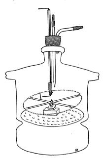
the kymograph, which of course also carries a suitable time tracing. Two other glass tubes through the rubber stopper allow gas or volatile liquids to be run in. An electrical contact is avoided in the recording mechanism because of the explosibility of several of the anesthetic mixtures.
