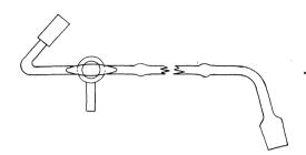
delivery tube of the chamber. After the upper cock of the Van Slyke absorption chamber has been closed this stop-cock may be turned to admit atmospheric pressure before detaching the delivery tube.
