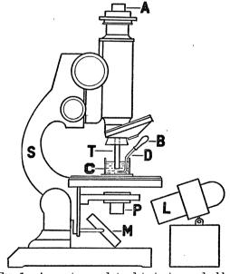
FIG. 1. Apparatus used to detect stream double refraction in virus-containing plant juices and other sols.
