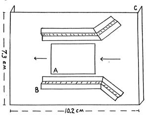
In preparing the film for use in the camera, old rolls of backing paper and film spools are obtained from the photographic supply house or from a developer of films. This is laid flat, black side down on a table and new numbers are placed about 26 mm apart in line with the old film numbers. These numbers should be spaced about 2 mm more apart than the length of the aperture A, to prevent possible fogging of adjacent film. Such spacing also marks off the exposures more clearly.
