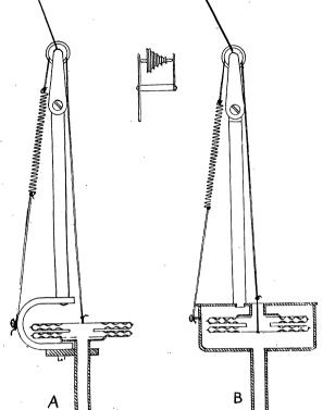
made to slide easily under the thread, it is possible to shift the position of the stylus while it is writing on the drum. The writing stylus may be replaced by a small mirror and a beam of light recording on a moving photographic strip.
