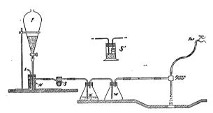
This crucible is placed in the specimen bottle (S). The replacing fluid in the Walter's special separatory funnel for single drops (F) is started dropping at the desired rate, the flow being regulated by the stopcock. The suction from the filter pump draws air from the inlet (I) through all the containers and
