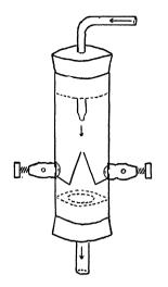
centimeters and about eight centimeters long was used. Two holes were blown opposite each other about six centimeters from one end of the tube. Through these holes were placed brass binding posts held in place by a screw from the inside. Small rubber washers were used to prevent breaking the tube on tightening these binding posts. Each screw head carries a length of platinum or non-corroding wire shaped as shown. These contact points are about one millimeter apart.
