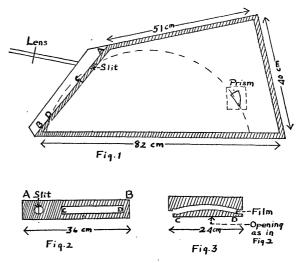
condensing lens and the quartz prism the only optical parts. The prism, which was cast by the Thermal Syndicate of Brooklyn, N. Y., has a front surface of 28 inches in radius, and makes an angle of 30°
