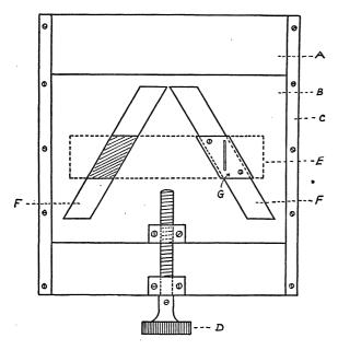
B which are placed in contact as shown in the figure. Plate B is kept in place by the guides C, and it may be moved over A by means of the screw D.
