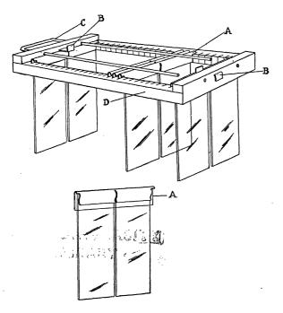
pendently of the others and apart from the two end clips serving as legs, as few or as many as may be desired can be put in up to the capacity of the rack. Any clip with its slides, except the end ones, can be readily removed for examination at any stage of the staining process without disturbing the others. If desired, all the clips in the frame can be secured against falling out when the rack is in any position
