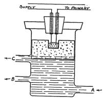
tecting water-cooled X-ray tubes from failures of the water line, the operation of which depends on the outflow from the tube. A device actuated by the water flowing out of the X-ray tube was constructed by the author and used at Cornell University in 1926–1927. Inasmuch as the arrangement used is much simpler in construction than the one described in the journal, and quite efficient, it seemed worth while to give its description here.
