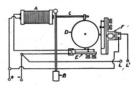
was rewound with No. 30 B & S enameled copper wire, and the connecting wires on the chronograph were rearranged in such a manner (see Figure 1) that the pendulum is driven by a shunt from the main source of current. In order to meet our needs for time magnets at fifteen or twenty desks a 24-volt storage battery and a rectifier were installed, and the bobbins of the Harvard signal magnets were rewound with No. 38 B & S enameled copper wire.
