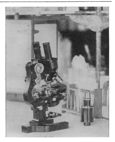
CDE-18 Research Microscope is equipped with 16 mm and 4 mm Apochromatic Objectives, 2 mm Apochromatic Oil Immersion Objective, 7.5x and 12.5x Compensating Eyepieces, monocular body tube for photomicrography, circular revolving stage with mechanical movement in two directions, complete substage actuated by rack and pinion and Aplanatic Condenser 1.40 N. A.
