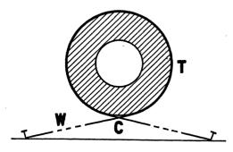
necessary to locate the cut exactly some kind of clamp or guide should be used until a groove is started. If a deep cut is made the point "C" where the wire crosses causes binding. When this stage is reached it is well to mount the tube in a lathe and hold the wire in the groove using only one half of a turn. (Be sure to protect the lathe from the compound.) New wire should replace the old frequently to avoid binding when the new is used.
