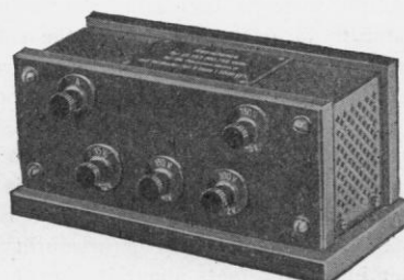
Cat. No. 560024 Combined Multiplier. Ranges: 15, 150, 300 and 750 volts. Resistance 1000 ohms for every 3 volts.
