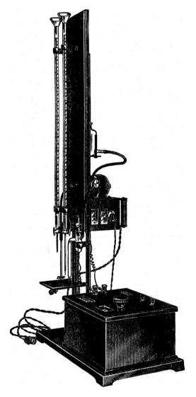
Adapted to the determination of end-points either by observing a sudden deflection of the galvanometer as in the titration of dichromate with ferrous sulfate, or by plotting readings proportional to electromotive force against volume of reagent.
