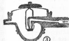
Now let's shut the outlet. The incoming gas will lift the diaphragm and make the seat close the nozzle. This prevents any more gas from entering.
