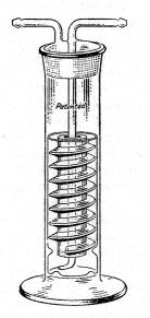
they escape at the surface. The liquid circulates upward with the bubbles and then downward both through the center of the spiral and around the outside of the shield.
