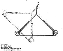
The advantages of the gauge are that a minimum of mercury is required, less space is taken and perhaps most important there is no exposed surface of mercury.
