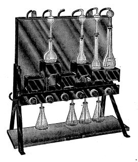
This distilling outfit is arranged in such a way that flasks of almost any size or style may be used as the heaters are adjustable for height. As illustrated, the battery of heaters is supplied with individual snap switches so that any or all units may be used independently. If desired, the snap switches may be omitted when all the heaters will be in operation at one time. This arrangement reduces the cost slightly.
