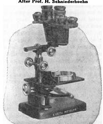
This microscope is most useful inasmuch as it is constructed to serve in an ideal manner for the determination and calculation of ore-dressing products. Being a microscope for binocular vision it renders a stereoscopic effect combined with an extremely large field and long working distance between specimen
