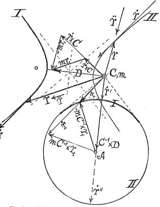
The hyperbola II (light lines) and the remainder of the hodograph belong together and these correspond to an attracting mass at m. Consequently the velocities are all relatively large with a maximum (dr/dt)'', again normal to D. All vectors through m originate there. The aim is along the asymptotes. CARL BARUS
