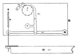
causes a downward pull of the lever (L 1) to which pawl (P) is attached, the ratchet wheel is turned the distance of one tooth, and the hand on dial 1 moved one space. A spring (Sp.) lifts the lever (L 1) to its former position after lever (L 2) has returned to the axle of the cage. The number of revolutions made by the cage are thus automatically recorded in figures which can be read at a glance.
