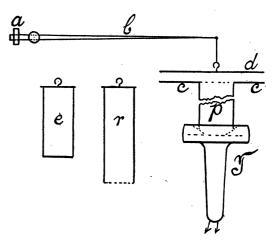
This is of course nothing further than a modified example of the familiar pneumatic paradox. When the pipe howls, the distance from which d may be attracted and held is perhaps 2 cm. beyond which the couche of diminished static pressure is ineffective. The thickness vanishes with the intensity of sound.
