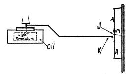
wire K attached to the end of an aluminum wire which is itself attached to the light pendulum by a flexible connection. The motion of the pendulum is thus transmitted to the mirror M which is cemented to the nickel wire at another point. The rocking of the mirror is recorded in the usual way on bromide paper.
