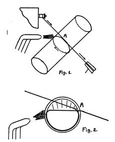
To insure success proceed as follows: Take a length of about one foot of nichrome wire, connect it up to a D. C. (or A. C.) dynamo current and include an adjustable tin resistance (for the current required must necessarily be large). The wire is held under tension by pulling on it with a pair of pincers, as shown in Fig. 1. Care must be taken not to let the two parts of the wire touch at A.
