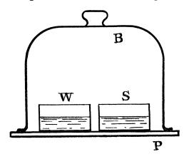
plate glass and B is a bell jar. For equilibrium the pressure of the vapor above S would have to be less than that above W. For this reason the water gradually distills from W into S.
