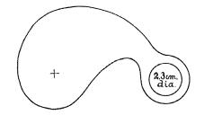
in diameter (a hair larger than the outside diameter of the standard eyepiece) is bored by means of an extension bit at one end of the screen. The distance from the center of this hole to the middle point of the broad wing of the screen is 8 cm. The extreme length and width of the screen is 12.5 cm. by 7.5 cm.
