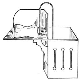
allowed to drop into the basket. This rod is ordinarily held in place by a nut, but it might be provided with a lock. It would thus be impossible to remove the towels by any one not provided with a key without tearing them.
