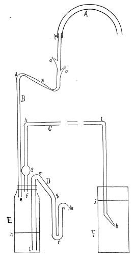
will in consequence be frequently interrupted.) The aquarium is represented by F and the surface of the water by j. In the bottle E, n represents the level of the water while running. The bottle E is fitted with an airtight rubber stopper with three holes through which the tubes A, B and C pass.
