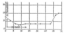
The method of investigation consisted in aspirating the air of the room continuously through the fog chamber and examining it by exhaustion from time to time. The result may best be given graphically by laying off the nuclei in thousands per cubic centimeter in a way to show their variation in the lapse of minutes of time.
