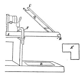
A, shown also in end-section at A', is a piece of wood two by two inches and about three feet long, grooved by means of a rabbet plane so as to clamp firmly to the lantern table (see A'). The arm B bears the two grooved strips C which carry at an angle of  $45^{\circ}$  the mirror D. This casts the image on the drawing surface E, where it may be traced with ease.
