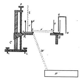
the drops issue. I have tried several arrangements of apparatus for the purpose, and have finally settled on one which is highly satisfactory. Reference to the figure will show the details of this, although not the proportions, as I have not had the parts drawn to any scale.
