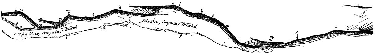
FIG. 1. Map of a zone of dislocation revealed at the surface after the earthquake in the Owens Valley, California, in 1872. Surveyed by Mr. W. D. Johnson, U. S. Geological Survey, in June, 1907. Scale, 240 feet equal one inch. The figures indicate throws, and the arrows the facings of the scarps.
