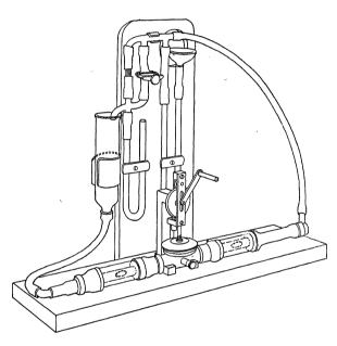
tric rim and rises and falls with the rise and fall in the rim of the plate. The motion of the small wheel is transferred through the yoke, rod and disk to the rubber membrane and thus to the interior of the ventricle.
