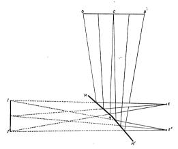
OCO' is the stereoscopic card. MN and NM' are the two mirrors. II' are the superimposed images of OC and CO', and E, E', are the positions of the two eyes.
