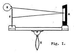
FIG. 1. The apparatus as seen from the side. E, the eye; C, the stereoscopic card; M, the mirror; H, the handle.
