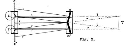
FIG. 2. The apparatus as seen from above. The letters as above: V, the combined view as projected by the eyes in stereoscopic vision; r, r and l, l, the paths of the rays in the right and left eyes from cards to mirrors and back.\*
