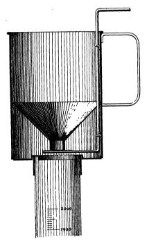
Without going into details, I may state that I obtained a very efficient regulation of the flow by adding to the funnel a movable stopper.\* By doing this I found by many practical demonstrations that it becomes immaterial as to with what rapidity, or in what manner, the funnel is filled before opening the stopper. This removes at once all source of error connected with the emptying of the cranial contents, and allows us to dispense with the extra vessel used in measuring the
