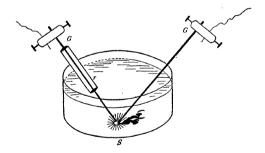
ends of the bars of metals, g, g, are brought sufficiently near that an arc is established between them beneath the water. The metal is torn off from the bars in such a fine state of division that it forms in the water a colloidal solution.
