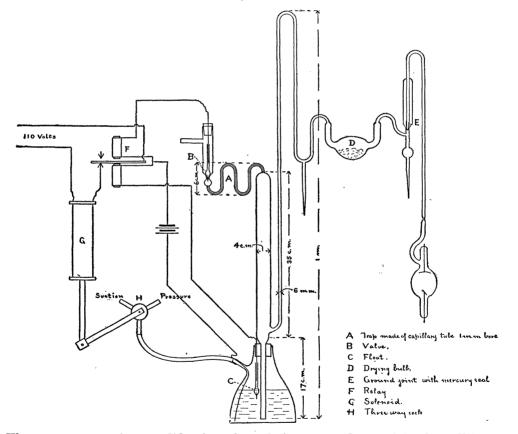
The pump proper is a modification of a common form of Geissler pump. It consists of a long glass tube, about  $1\frac{1}{4}$  inches in diameter, which has a mercury trap and a small glass valve at the top. The bottom of the tube is drawn down and dips into a
