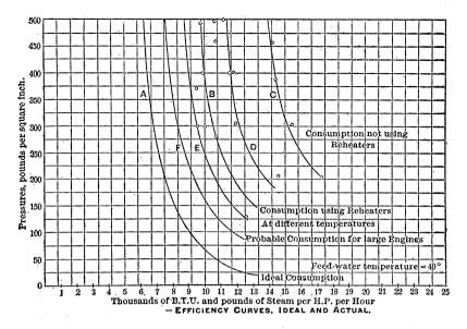
where the value of a varies from 18 on the line A, to 25 on B, 30 on C, and to 22 and 24 on lines F and E; w being weight of steam per h. p. per hour, p steam pressure.
