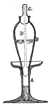
the tube B, to contain the heavy liquid in which the separation takes place, the stoppers C and D to close respectively the upper and lower ends of this tube. All of these separate parts have ground fittings, so as to be water-tight. The tube is so simple that no special explanation of the method of using it is needed. It will be seen that when the two stoppers, C and D, are out,
