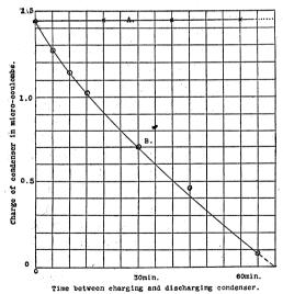
curves A and B in the accompanying figure. A was obtained under the ordinary conditions. B was obtained when the Crookes tube was in action, and placed about six
