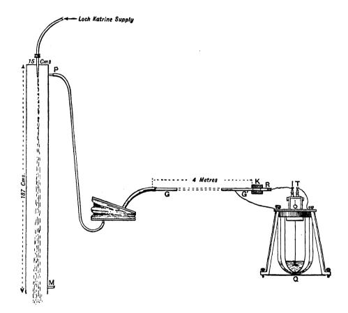
last Monday (March 25), we found .28 of a volt in 15 minutes with no obstruction to the shower; and 4.18 volts in five minutes, with a metal plate held three or four centimeters below the mouth of the funnel; the air being drawn from the upper outlet (P). Immediately after, with P closed, and air drawn from the lower outlet (M), but all other circumstances the same, we found .20 of a
