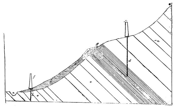
a, stream at foot of hill; bb, mass of maltha, asphaltum and rubbish; c, derrick of 1880; d, well of 1880; eec, barren sand stone strata; f, derrick of 1865; g, spring of water and maltha from oil-bearing strata pierced by well d, of 1880; h, well of 1865 in barren sand stone strata.
