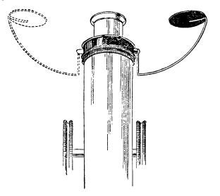
Another consists of a small plate extending horizontally from the cap of the ocular. In this the edge must be cut away to admit the bridge of the nose. This gives it a curved form, and prevents its being used before each eye alternately, except by removal and inversion. It must also be removed with each change of ocular. These removals and replacings demand so much time that most workers think it hardly worth the trouble.
