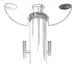
Another consists of a small plate extending horizontally from the cap of the ocular. In this the edge must be cut away to admit the bridge of the nose. This gives it a curved form, and prevents its being used before each eye alternately, except by removal and inversion. It must also be removed with each change of ocular. These removals and replacings demand so much time that most workers think it hardly worth the trouble.
